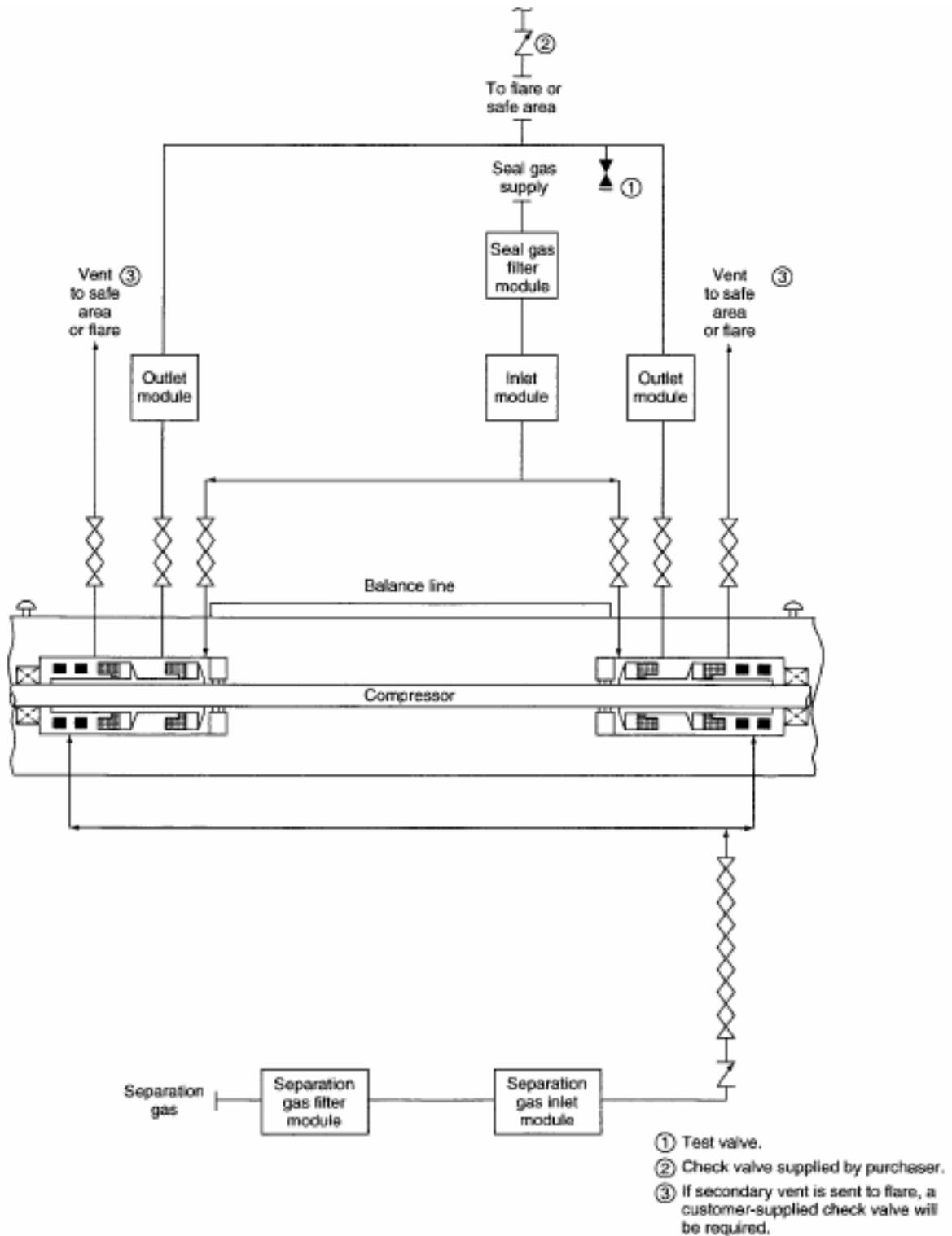
**Figure 4: Tandem Dry Gas Seals Support System Schematic**
