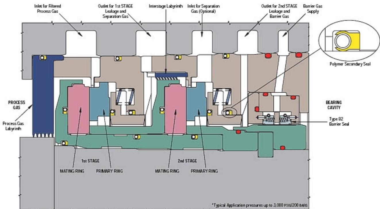
**Figure 3: Cross-sectional view of a Typical Tandem Gas Seal**
