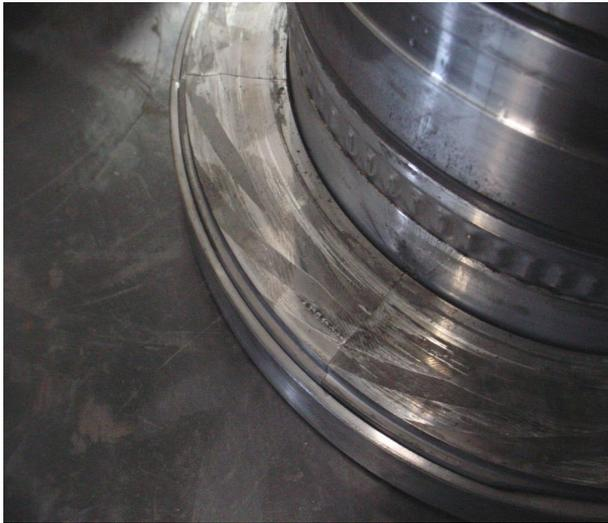
**Figure 7: Damaged Mating Ring**
