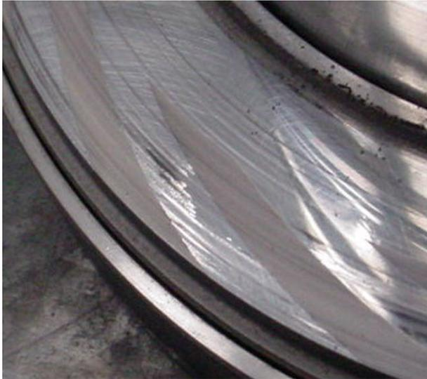
**Figure 8: Scratches on the Mating Ring**
