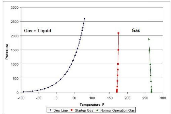
**Figure 9: Seal Gas Phase Diagram**
