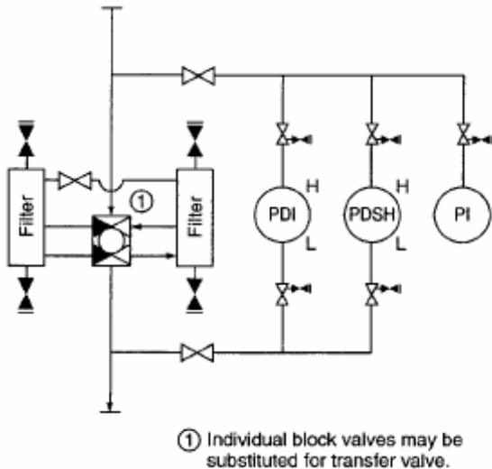
**Figure 5: Seal Gas Filter Module**
