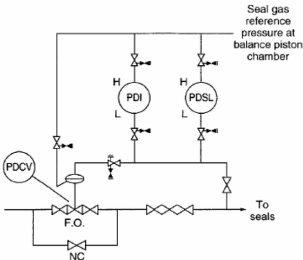
**Figure 6: Differential Pressure Control**
